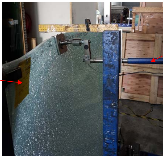
13.52 EVA Toughened Laminated Glass Panel
